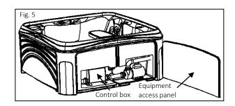
Power requirements 230 VAC, 1PH, 50HZ, 32 AMPS (40 AMP CIRCUIT BREAKER) 3 WIRE (LINE, NEUTRAL, GROUND)
